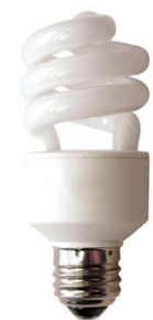
A CFL contains a mixture of argon and mercury gases that produces invisible ultraviolet light (UV) when the gas is excited by electricity.
