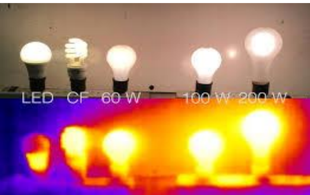
A CFL contains a mixture of argon and mercury gases that produces invisible ultraviolet light (UV) when the gas is excited by electricity.
